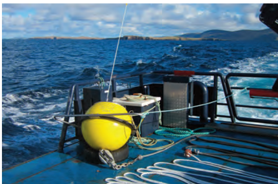
Waverider buoy measuring wave height and frequency Image courtesy of Alan Bourhill
